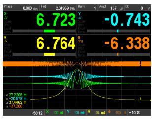
Large numeric readout with strip chart recording
